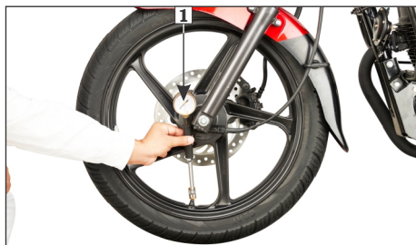
(1) Air pressure gauge
