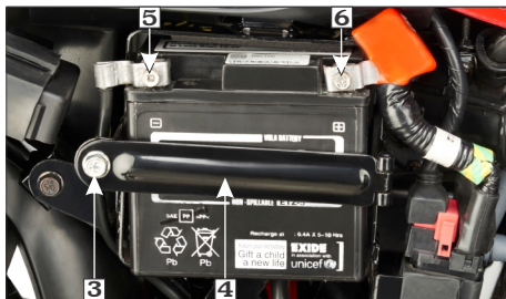
(3) Bolt (4) Battery clamp (5) (-)ve terminal (6) (+)ve terminal
